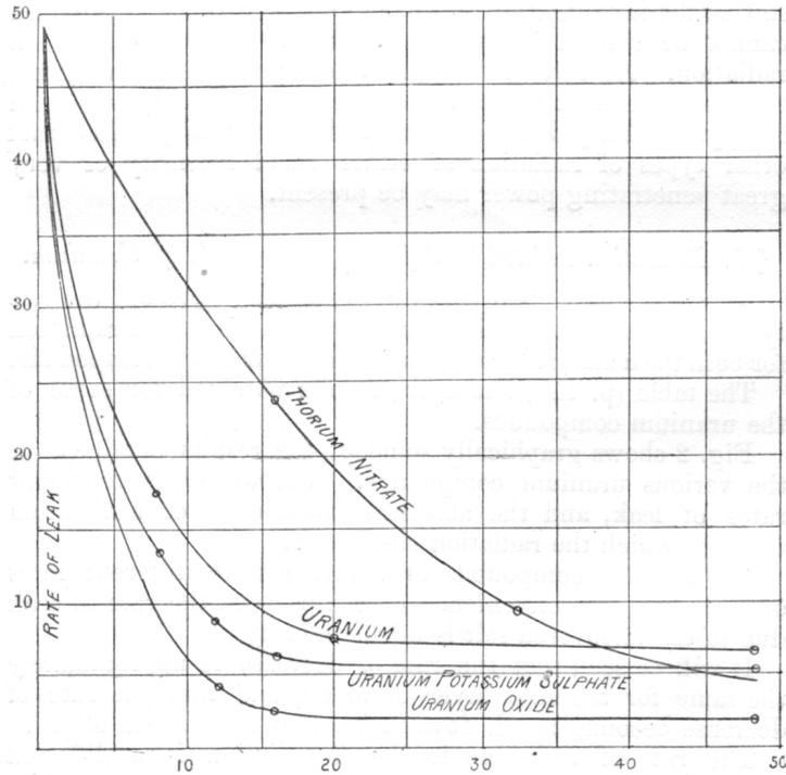
Figure 2: Thickness of aluminium: each division 0.00012 cm.
